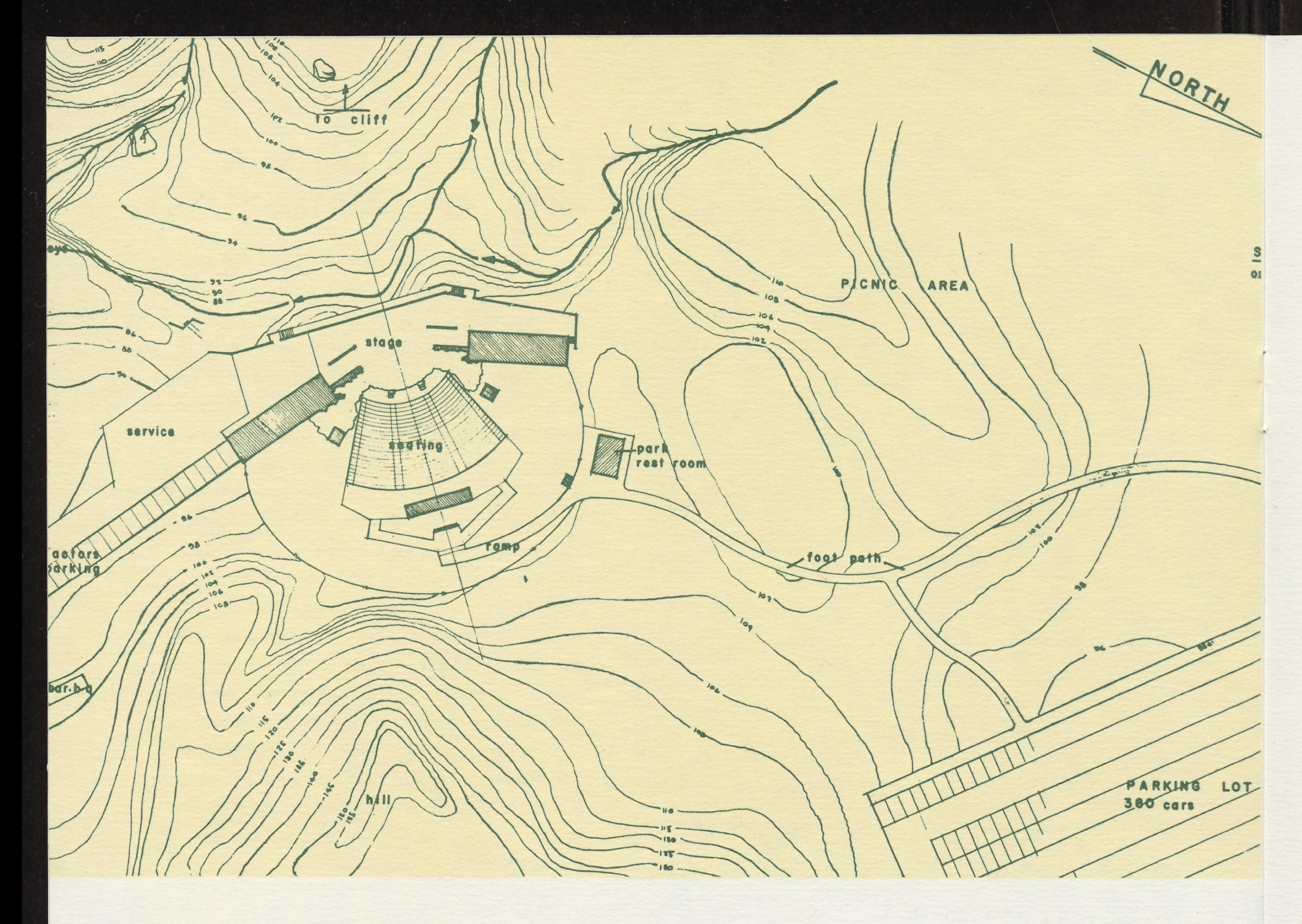
A scale drawing of the Architect's plot plan for the amphitheater in Palo Duro Canyon. The stage will lie within the contour of a 600-foot bluff which will serve as the backdrop. The cost of the theater and development of symphonic drama for the Panhandle will be \$350,000.
