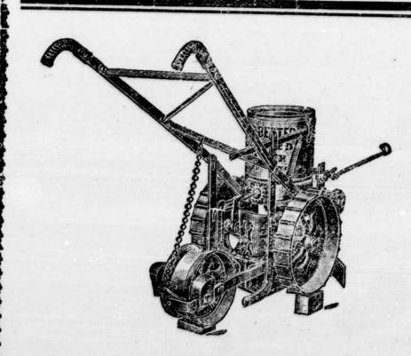
Plants Cotton one seed at a time. No skips no bunching. Plants a peck or more to the acre one to six inches apart, always one seed at a time. Saves half the work and labor in chopping. Positive force feed means absolute regularity of drop without cracking or crushing the seed. Each plant has room to grow, though chopping be delayed.
