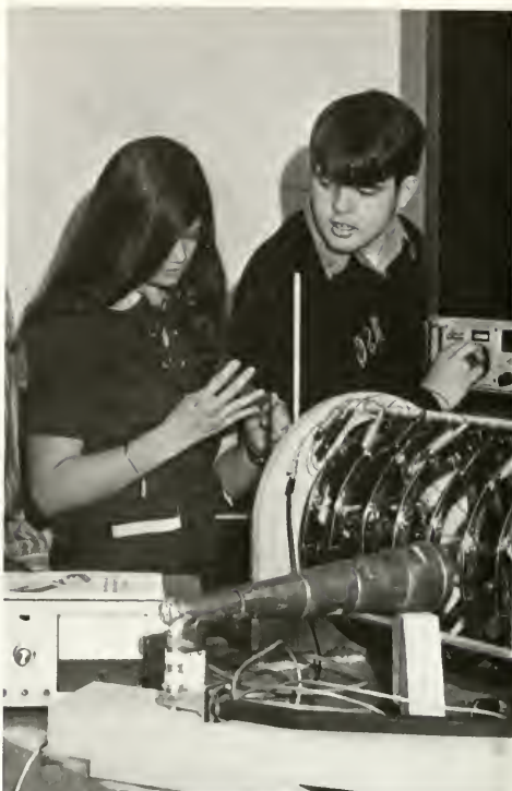
Michael Compton and Colette Hayes examine a single-wire transmission plasma device.
