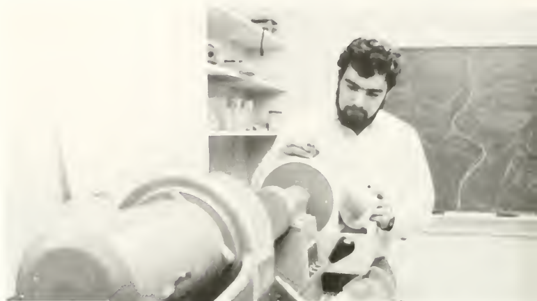
Ron Crowson, the president, tests soil samples in thin section machine in Geology Department.
