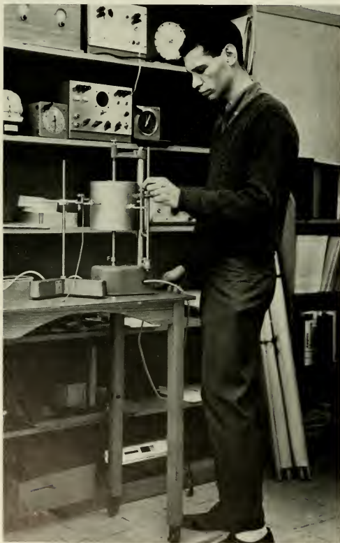
The galvanometer measures the presence of an electric current.
