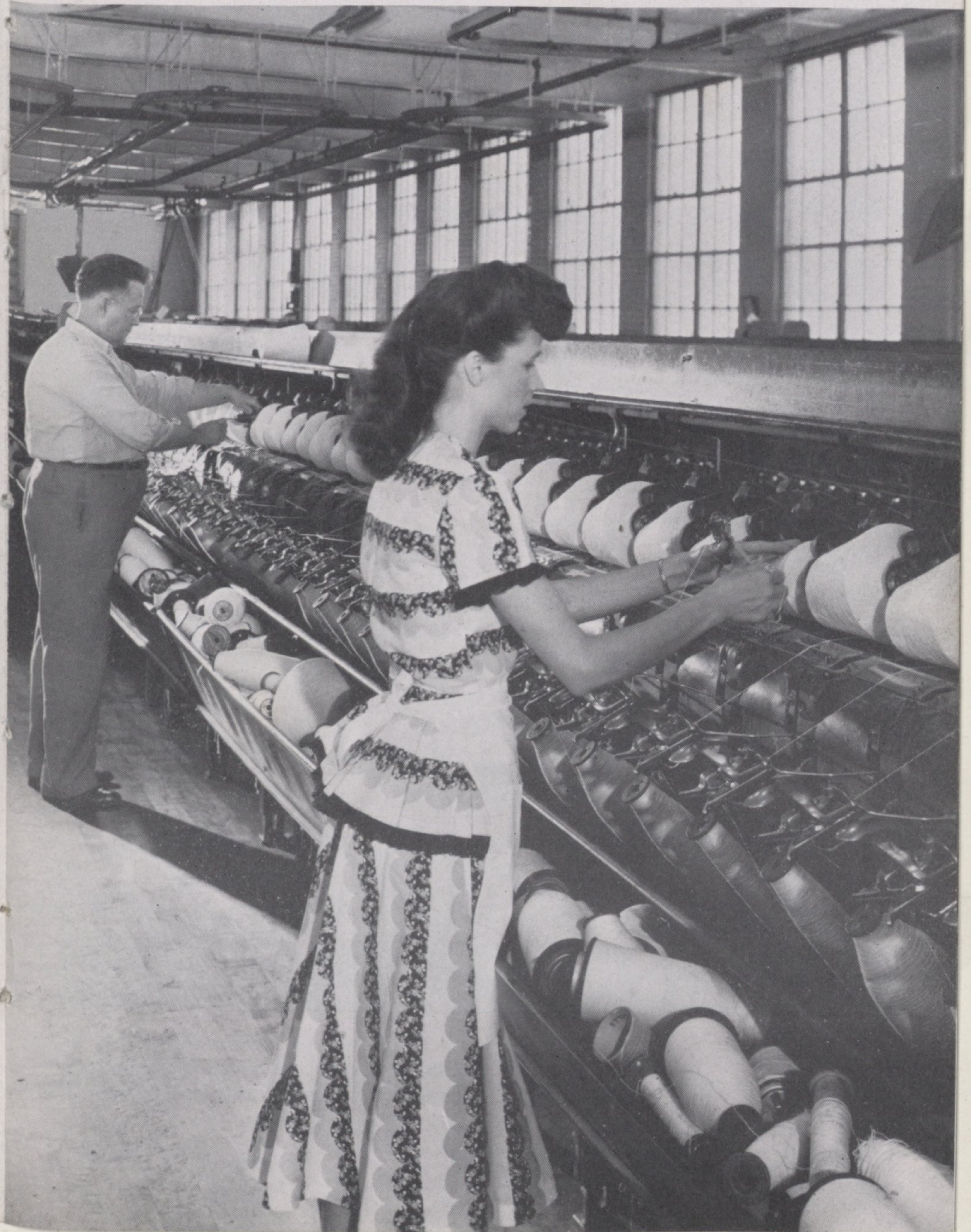
MARY LOUISE LANGSTON, nine years service, runs a high speed winder to transfer plied yarn from twister bobbins to cones or other type packages as requested by customers. WILLIAM DAVID HOWELL, mechanic, twenty-seven years service, adjusts a part on the machine.
