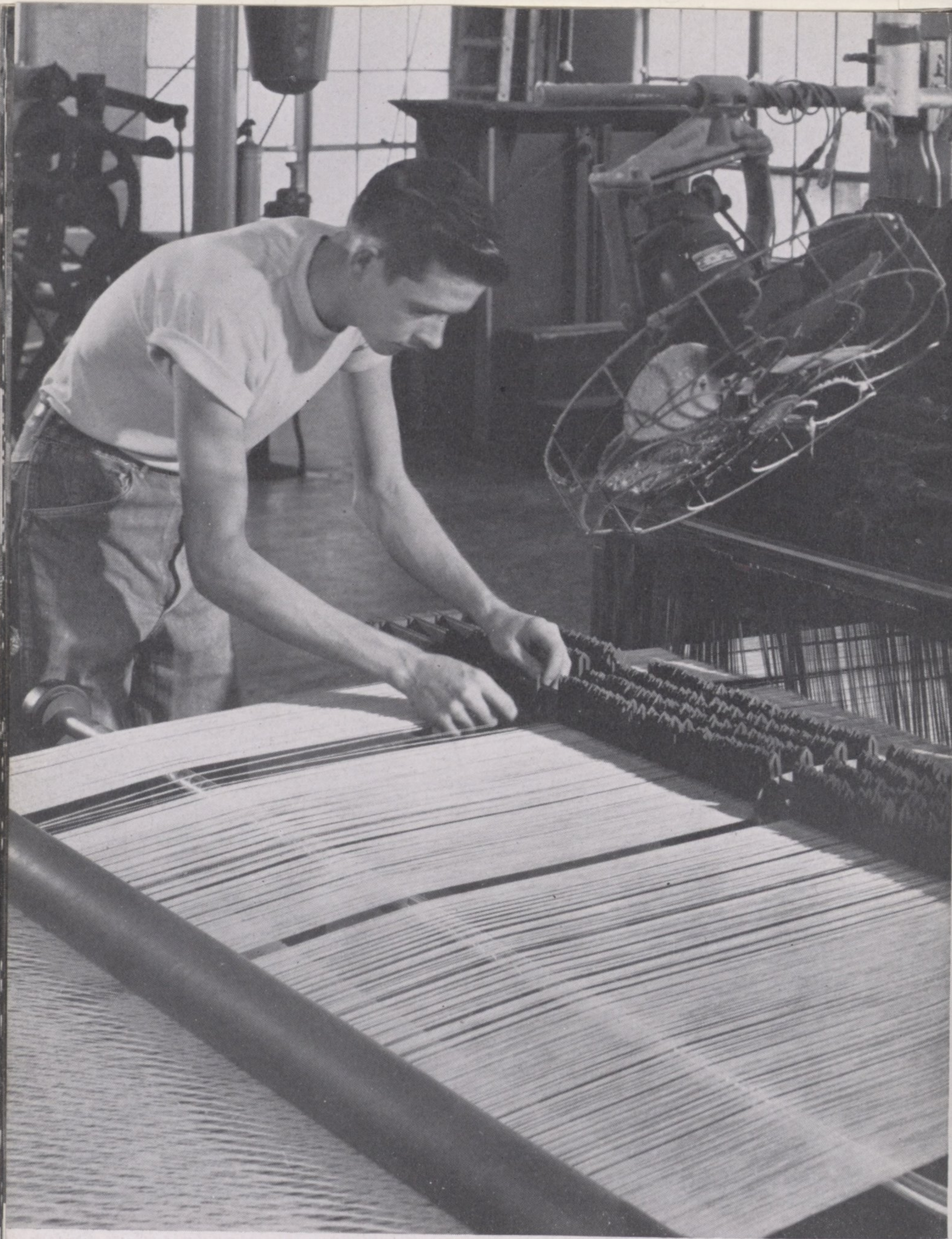
LEWIS CLIFTON WOOD, six years service, reties broken yarn ends on a warper. Hundreds of strands are drawn from cones and wound side by side on a huge spool, or beam, which will go into a loom in some customers weave mill.
