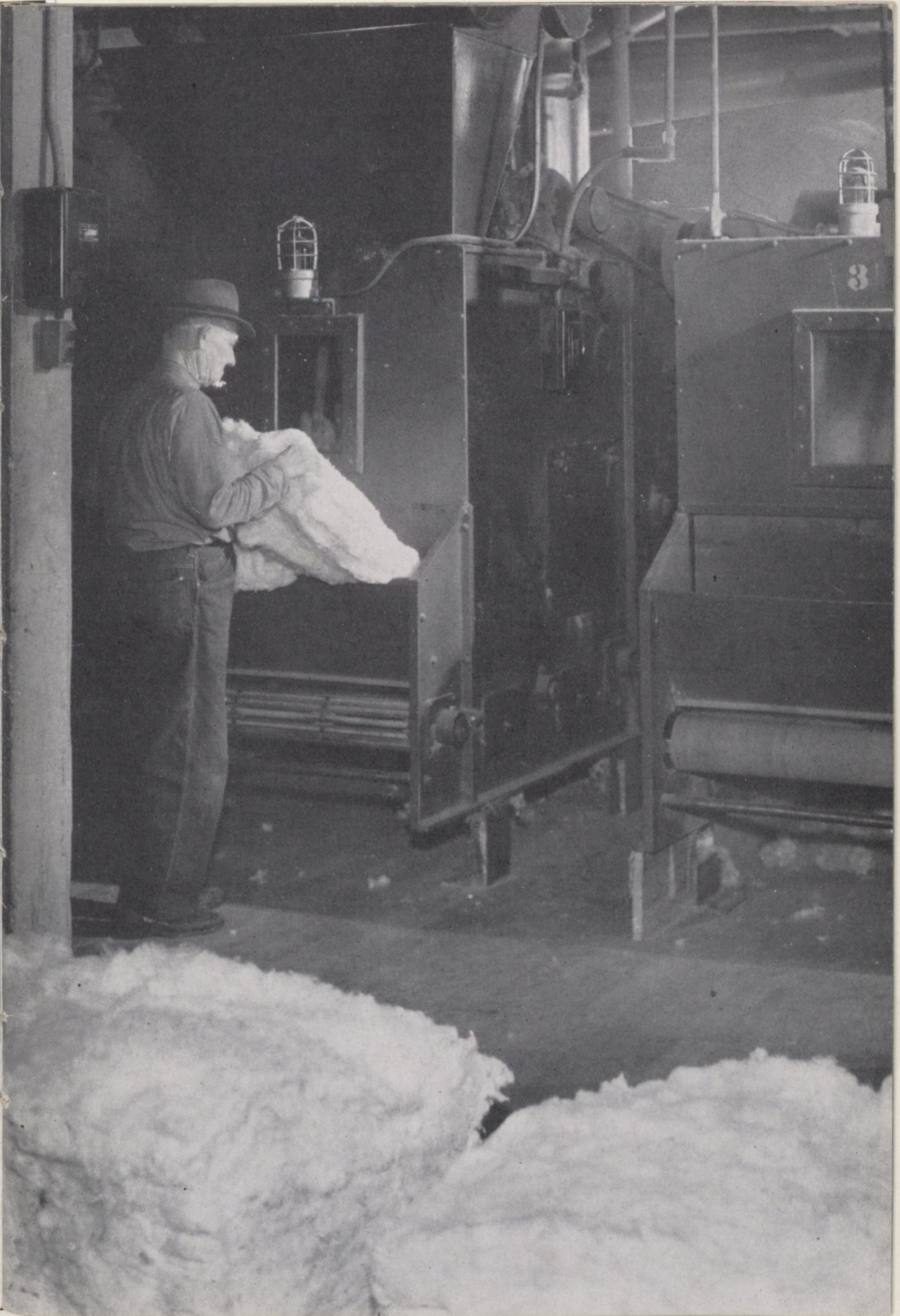
JONATHAN CLEE EDWARDS, seven years service, feeds cotton into an opening machine which starts the process of mixing, blending and cleaning the fibers. →
