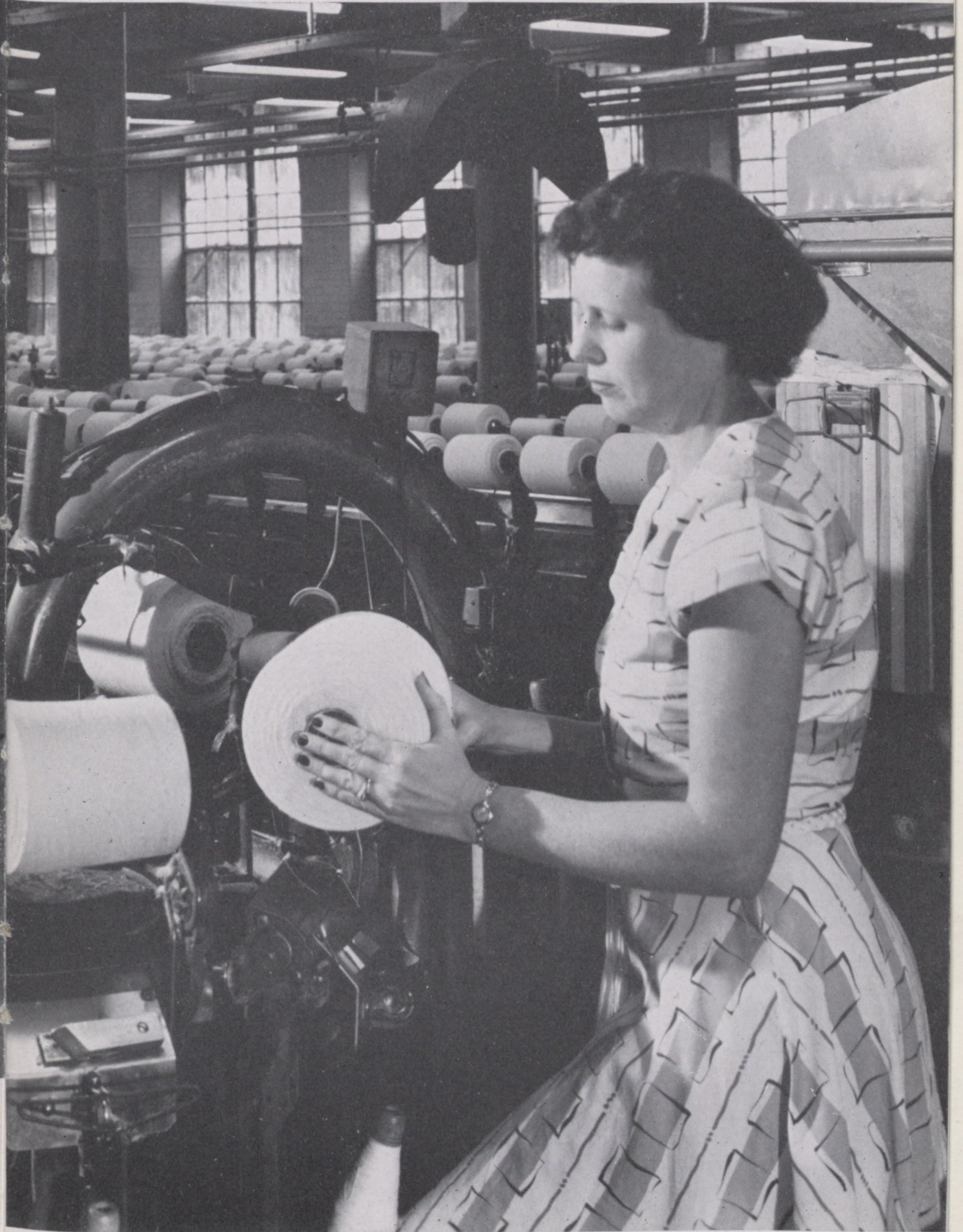
RUTH WILLIAMS HOWELL, seventeen years service, tends an automatic winder. This complex machine automatically ties and winds yarn from a spinning bobbin to a large tube for ease of handling in the next step.
