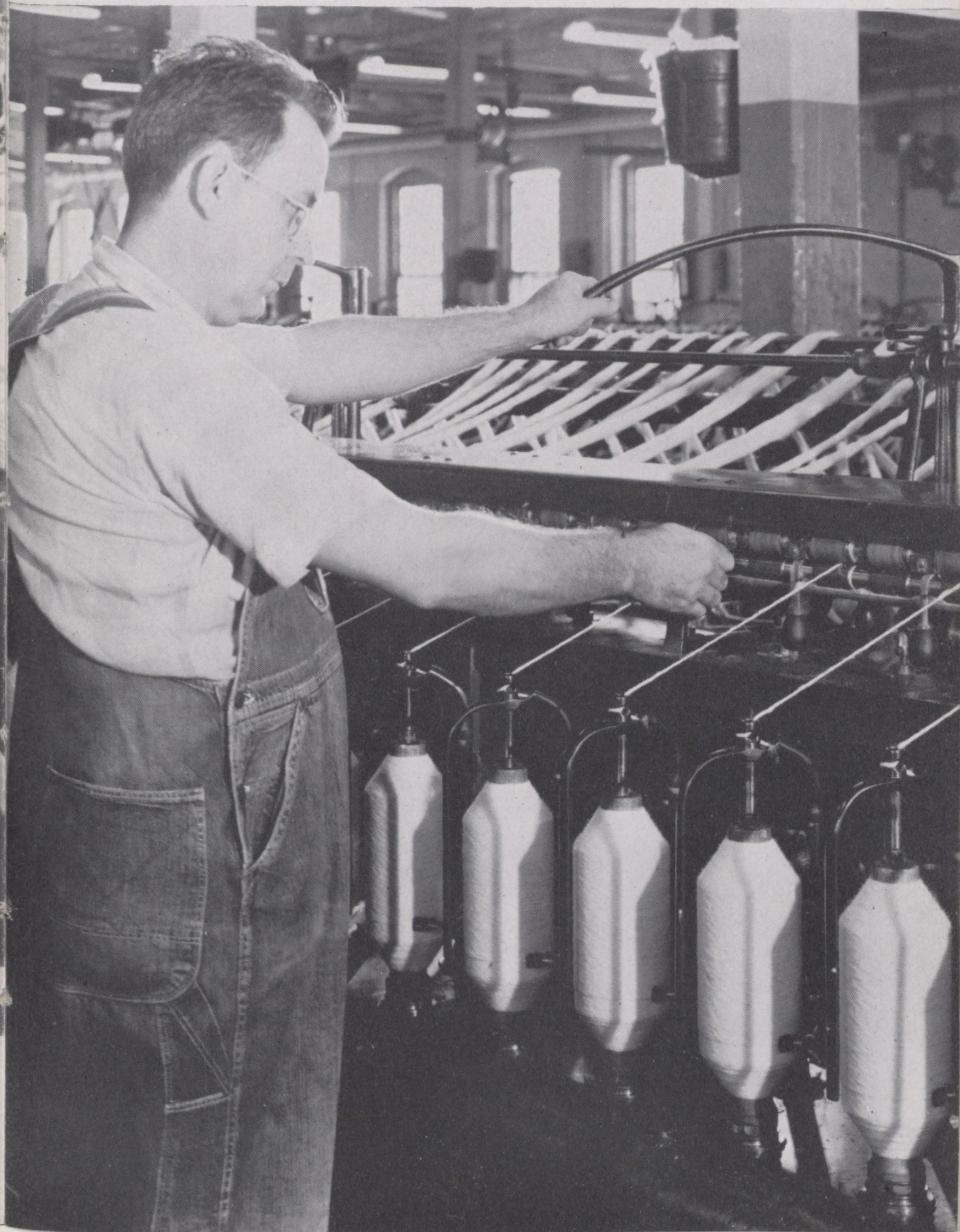
TOMMIE LEE THOMPSON, twenty-five years service, operates a roving frame. Drawing sliver is drafted between rollers to reduce it into a finer strand called roving. For strength the roving is twisted slightly as it is wound on bobbins.
