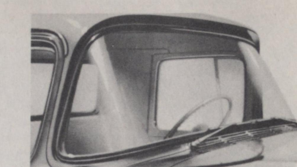
PANORAMIC VISIBILITY. A wide, wide windshield with over 1000 square inches of safety plate glass. Big-size door windows with glass-guard moldings, and a broad rear window, provide a sweep-sight view all around for safer driving. Curved, Full-View rear window is standard on the Iuxurious Cameo-Carrier, optional on other Task-Force cab models.
