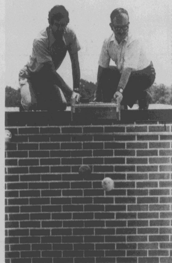
SHOTPUT WINS BALL RACE . . . Dr. Byron Coulter and Dr. Carl Adler, East Carolina University physicists, re-enact Galileo's Tower of Pisa experiment by using a shotput, a rubber ball and a specially constructed release gate that enabled them to drop the objects, simultaneously, from the top of an ECU dormitory. The white colored ball on the right is the shotput. (ECU Physics Department Photo.)
