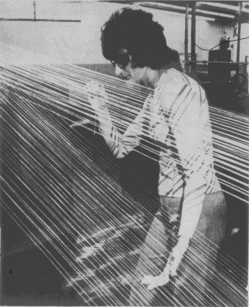
JUST STRINGING ALONG —A woman worker positions strands of fiber glass textile yarn to make them ready for feeding into a warping machine at PPG Industries' Lexington, N.C. plant. In textile yarn warping operations, several hundred strands of fiber glass yarn are
